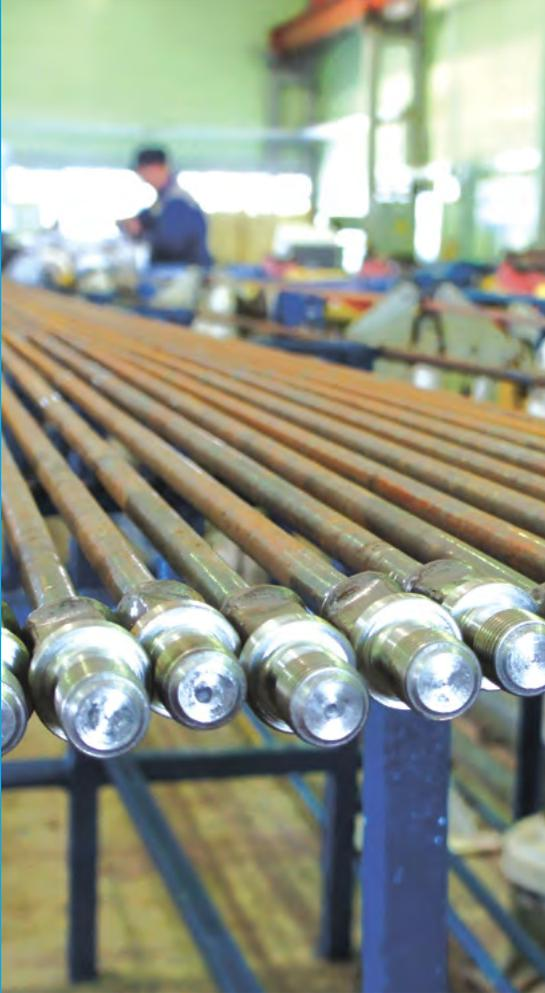
Pump rods of TMC group are produced on modern imported and home equipment made of highquality alloy steel with method of arc melting. At that chemical composition is chosen in such a way that physical and chemical properties of rod such as ductility, impact strength, fatigue strength, wear and corrosion resistance are balanced for use in wells with abnormal geologic and technical conditions.
