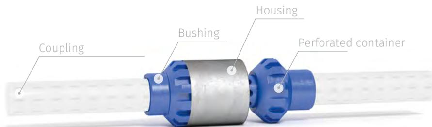
The coupling, like the scraper housing, has grooves for the fluid passage and centering in the column. The bushing freely moves between the coupling and the housing. The bushing has sharp edges for cutting deposits of salts and fibers of cementing materials from the inner surface of pipes. All waste is accumulated in a perforated container which is cleaned mechanically at the wellhead.
