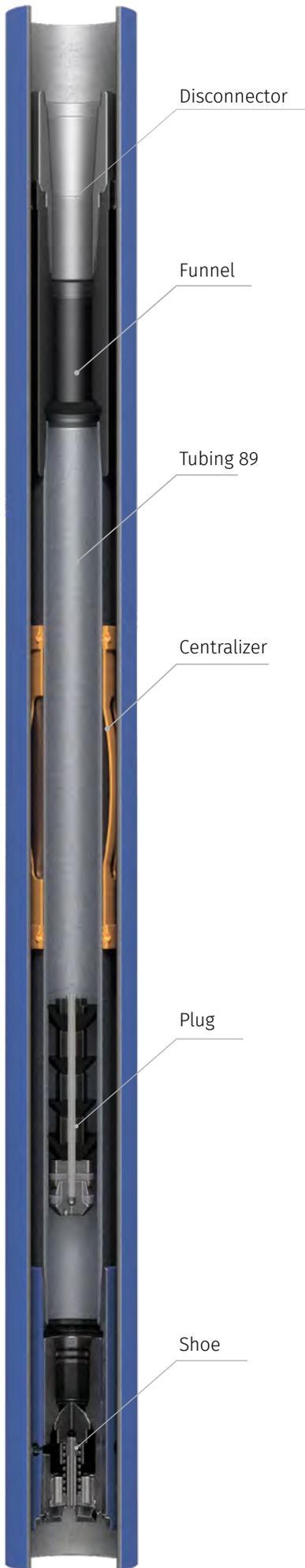
**Plug** is designed for separation of cement slurry from the displacement fluid, cleaning of the casing pipe wall from cement slurry residues.
